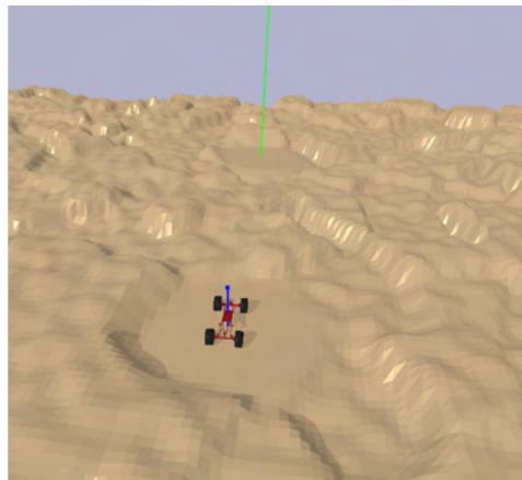
Fig. 5. Off-road driving simulation. In this task, the robot must reach the target indicated by the green laser.
