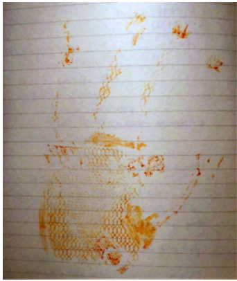
Fig. 3. Ink test used to determine optimal sensor placing.
