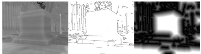
Fig. 5. Example of a thermal image (left), its edge map (middle), and its attraction field map (right).
