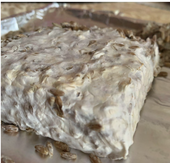
Fig. 4. Mycelial Bio-foam with rye-berry substrate
