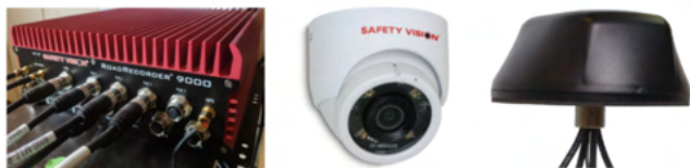
Fig. 4. Hardware components located on the bus (from left to right: onboard computer, exterior camera, GPS and network antenna).
