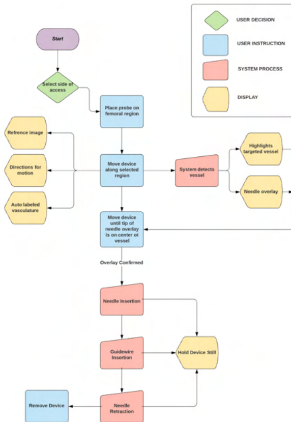
Fig. 2. Proposed workflow based on user requirements for the robotically assisted femoral vascular access device.
