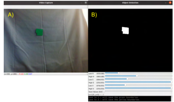
Fig. 4. Calibration Stage. A) Input image without any filtering, B) Image after a simple HSV filter for calibration has been applied
