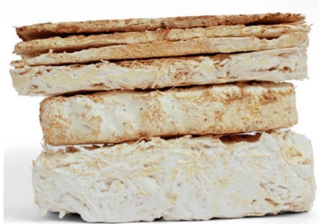
Fig. 1. Typical Structure of Mycelium-based foam [1]
