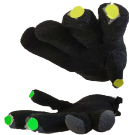
Fig. 2. Gloves used for interaction with AlgeGloves. Students wear a pair of gloves which have three colored circles each one in one finger: thumb, index and middle finger.
