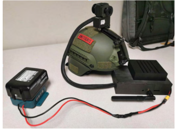
Fig. 4. Our own VIO setup. From left to right, the devices are: battery, helmet with fisheye cameras and IMU, Xavier.
