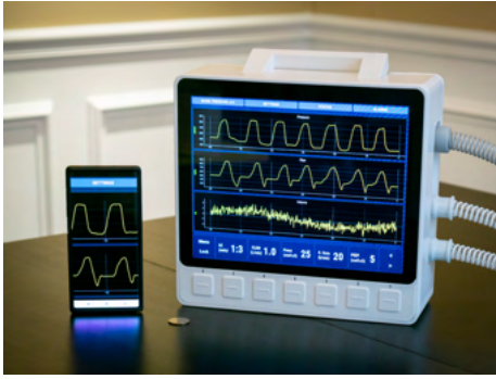
Fig. 2. RoboVentilator Device with Digital Monitor Displaying Pressure, Flow, and Volume
