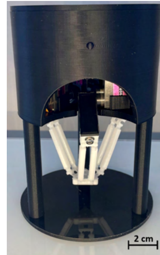
Fig. 1: The mechanical design of DeltaZ. The upper part of the robot encloses all motors and electronics and is supported by a tripod base. The 3D-printed soft delta component (white) has flexible joints that enable the robot to move similarly to a rigid robot.
