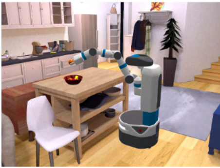
Fig. 5. A mobile Manipulator (Fetch Robot) in Habitat 2.0 performing rearrangement tasks. Taken from Figure 1. of Habitat 2.0 paper [20]
