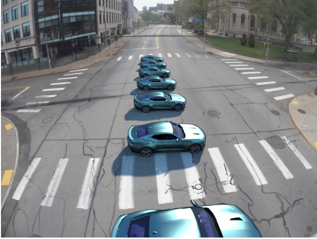
Fig. 3: Demonstration of our method’s geometry, perspective, and size consistency as a result of using an estimated road plane equation and camera parameters. The same car model has been rendered and inserted at constantly increasing distances from the camera.
